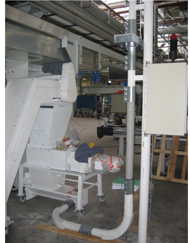
➤ Dry machine suction unit with chips crusher
