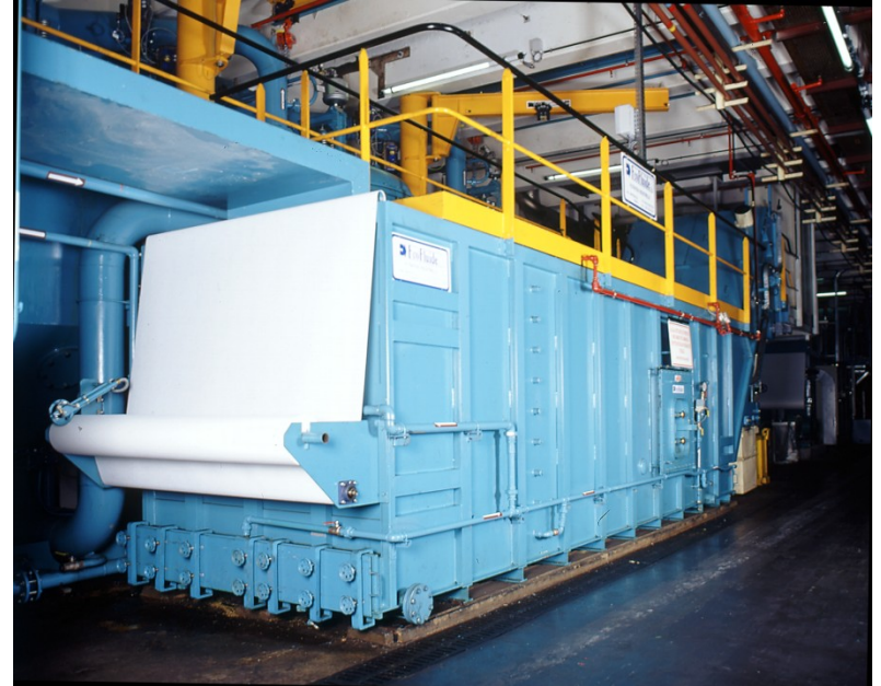
➤ The Vacuum Filter with Paper belt
