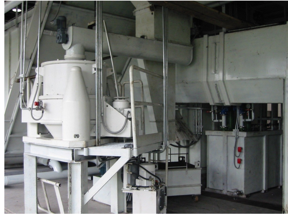
➤ The wringer: for chips treatment
