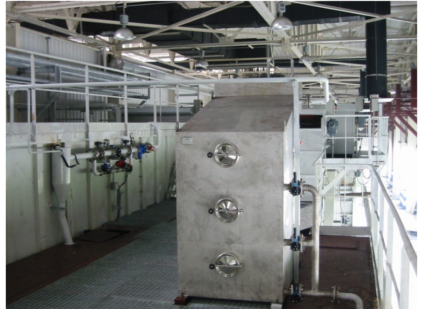
➤ The De-oiler: for separating the oil and water for recovery using.
